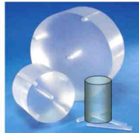
B. Cylindrical PMMA phantoms (Toth and Strauss, TS)
